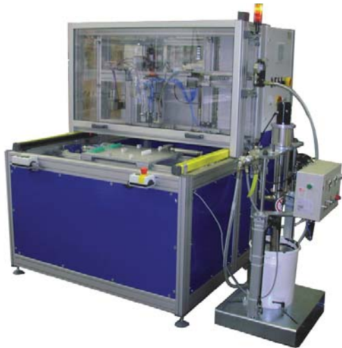
MiniTec Profile System is used extensively on specialised machinery such as this glue dispenser
