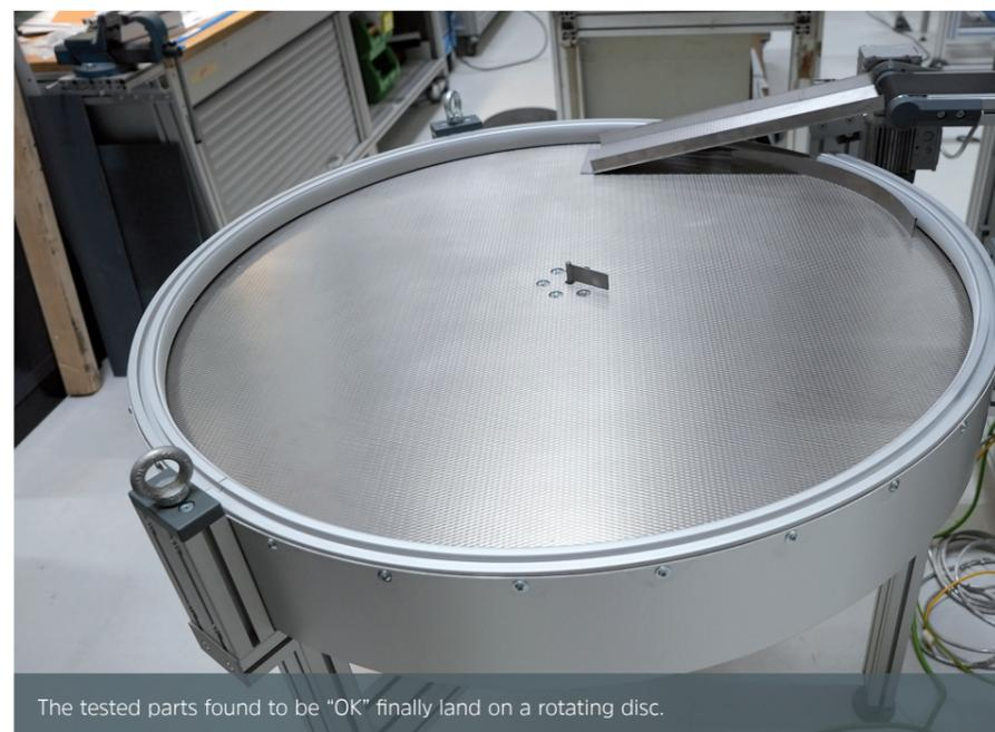
The tested parts found to be "OK" finally land on a rotating disc.
