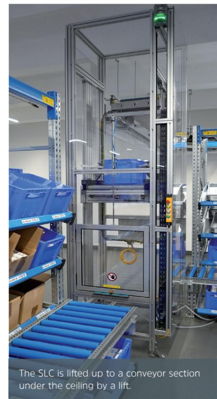
The SLC is lifted up to a conveyor section under the ceiling by a lift.
