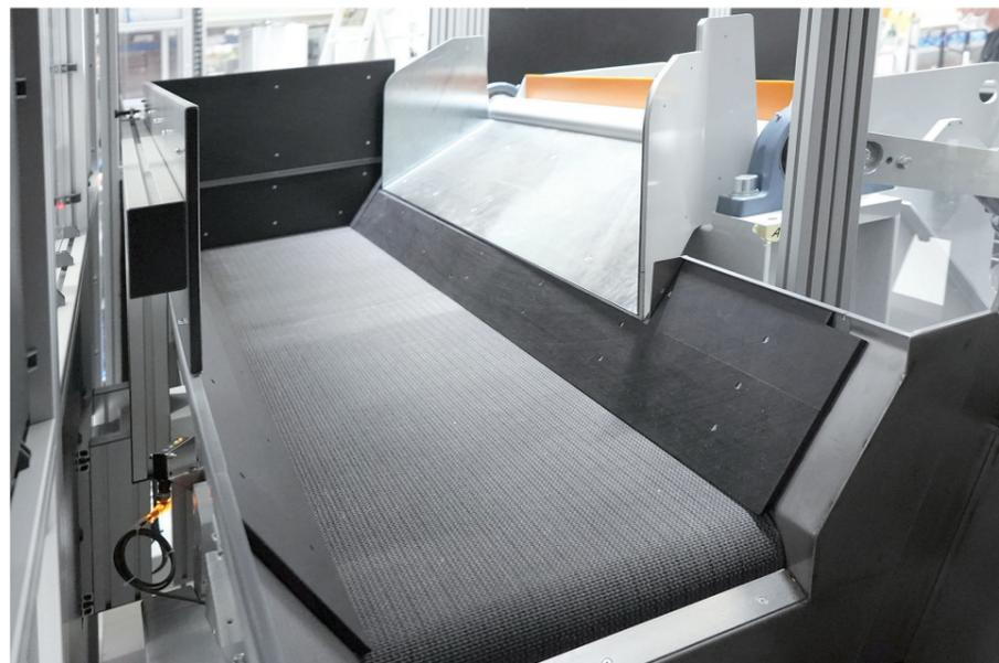
From here, the parts are carried by a conveyor belt to a step conveyor.
