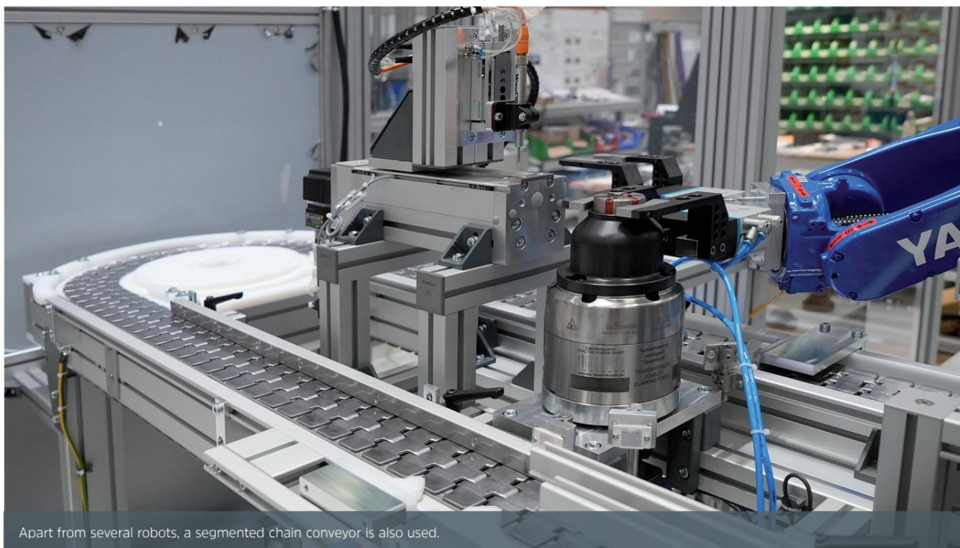
Apart from several robots, a segmented chain conveyor is also used.
