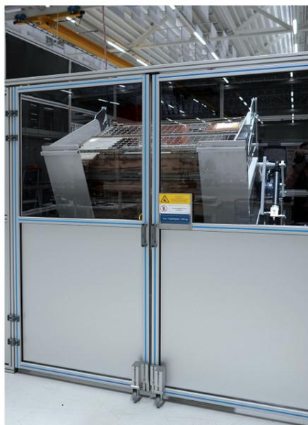
The products are tipped into a chute at the start by a tilting-inclining device.
