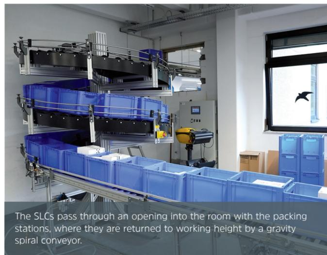
The SLCs pass through an opening into the room with the packing stations, where they are returned to working height by a gravity spiral conveyor.
