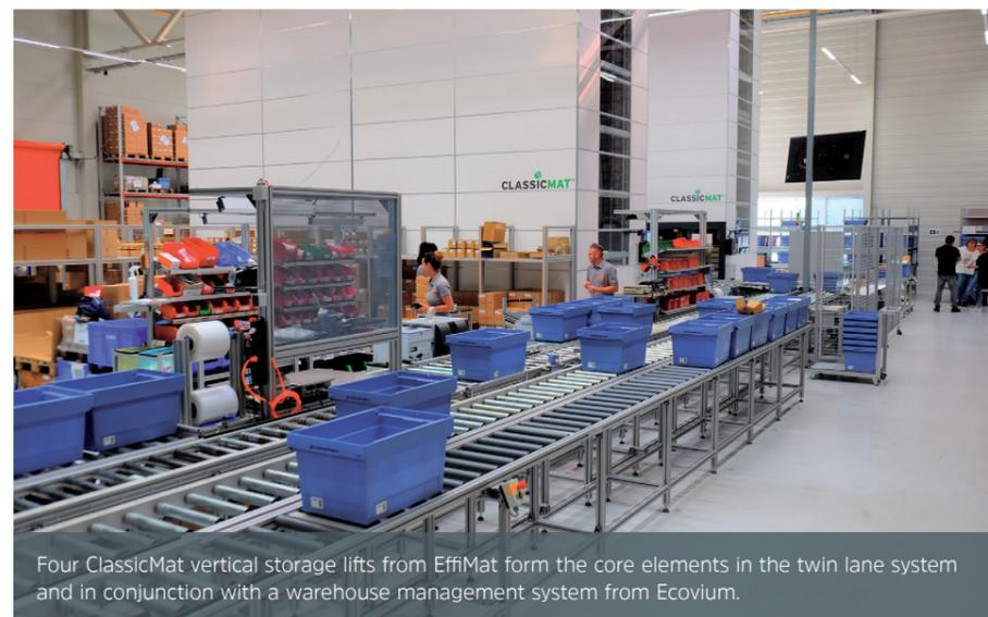
Four ClassicMat vertical storage lifts from EffiMat form the core elements in the twin lane system and in conjunction with a warehouse management system from Ecovium.
