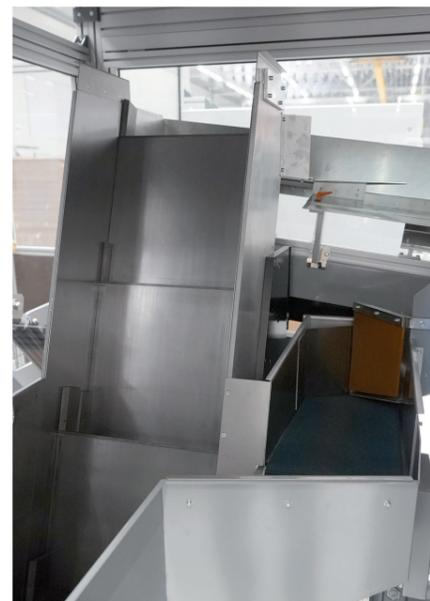
The step conveyor transports the parts upwards.
